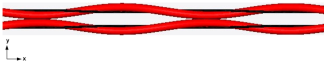
FIG. 3. (Color online) Textile application—pores open under tension in a complementary pair of HAYs.
